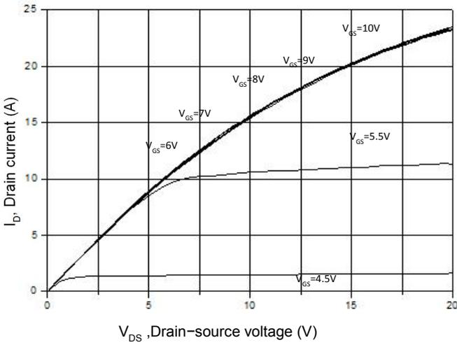
Figure 2. Transfer Characteristics
