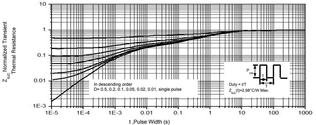
Figure 16. Transient Thermal Impedance, Junction to Case, TO-220/ TO-262/TO-263
